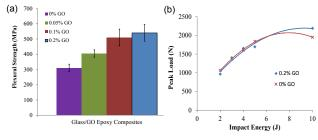
Figure 5: Summary of the mechanical characterization tests (a) flexural strength, (b) low velocity impact response.
